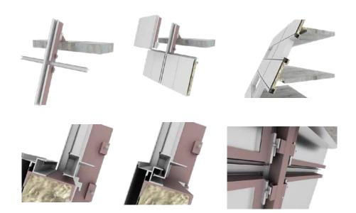
Top The building's south façade during erection. Above the 31st floor, the mechanical level that typically tops a residential high-rise is incorporated into the top of the pyramid. Façade openings that reveal terraces below become vents for the building's systems at this level. Above Diagrams from an Enclos PowerPoint presentation illustrate installation of the south face's vertical gutters and façade megapanels.
